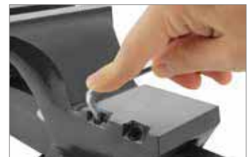
Adjustable spindle guides for backlash-free operation.
