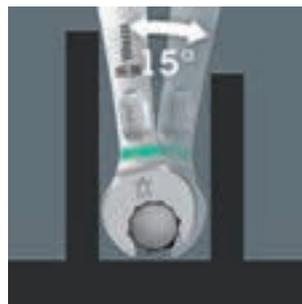
The Joker 6003 ring spanner with its special mouth geometry – mouth side pivoted by 7.5° and the double hexagon profile – doubles the placement possibilities when repeatedly turning the wrench 180° around the longitudinal axis. Bolts and screw heads can be "accessed" every 15°.
