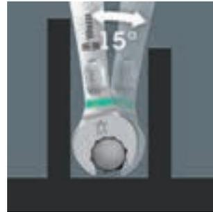
The Joker 6003 combination wrench with its special mouth geometry – an open-end offset by 7.5° and the double hexagon profile – doubles the placement possibilities when repeatedly turning the wrench 180° around the longitudinal axis. Bolts and screw heads can be "accessed" every 15°. The Joker 6003 will automatically find the respective placement point after every turn.
